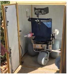
Rear wheels must be removed before storing. Wheels are easily removed/attached by pulling the quick release pin.
